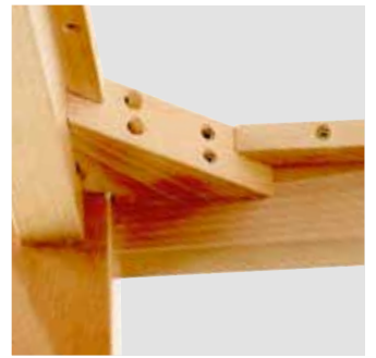
Extreme Table Joint Construction
